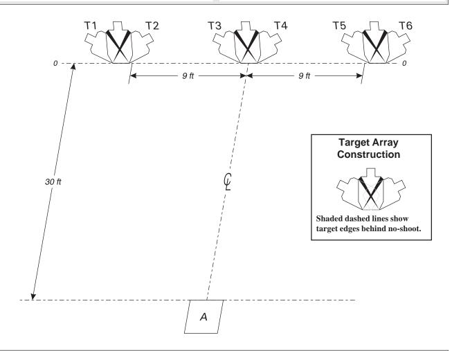
**SETUP NOTES:** Set no-shoots to 4 feet high at top of B-zone. Build target arrays so that the upper corner of the waist meets the lower corner of the no-shoot,
