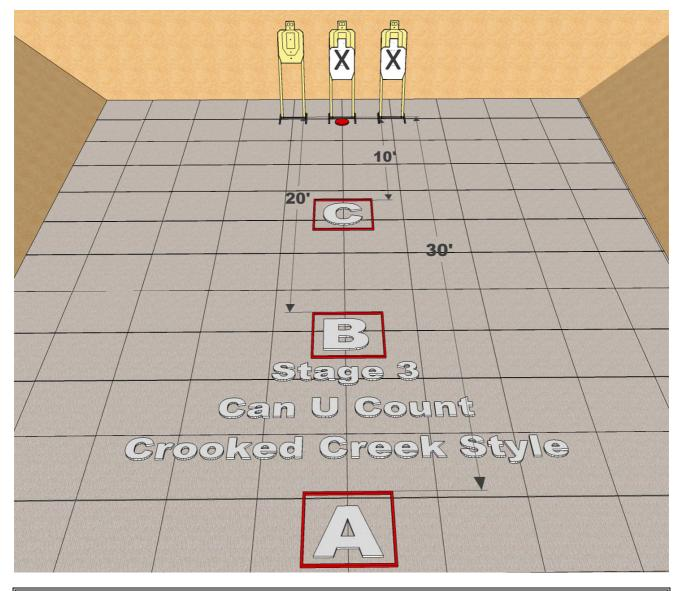
**SETUP NOTES:** Use the grid on the diagram. Targets are 3' center to center. Set inside front edge of shooting boxes to distances shown.
