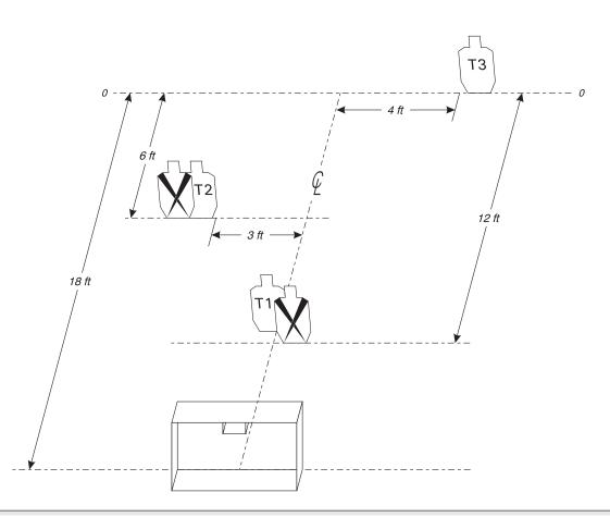
**SETUP NOTES:** Set paper targets to 5 feet high at shoulders. The "counter" can consist of saw horses. The shelf can be an opened cardboard box nailed to the underside of planking or boards. Have a replacement handy. Counter is 4 feet high by 8 feet wide by 2 feet deep.
