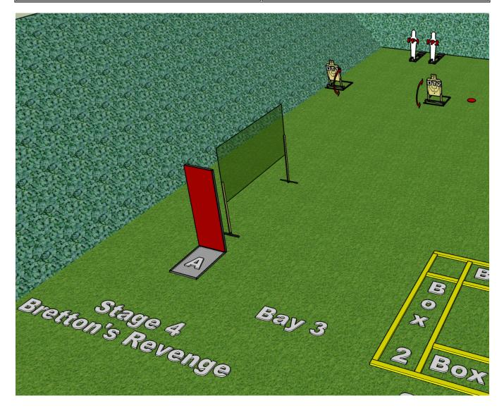
**SETUP NOTES**: Barricade is at least 24' from steel. DT1 & ST2 are at least 3 yards in front of steel. Position wall to prevent shots on both Peek-A-Boo targets from one side of barricade.
