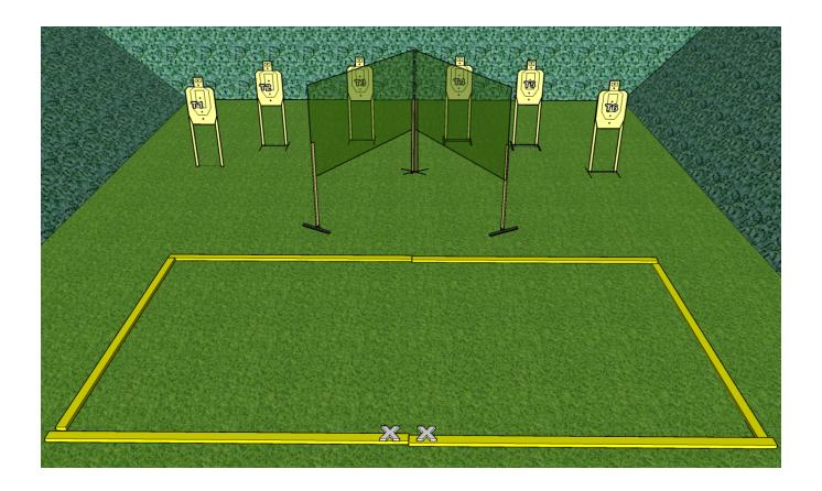
**SETUP NOTES:** Shooting area is 2 - 8' Fault Lines wide and 8' deep. Set walls at least 3' from front Fault Lines. Set end of walls 8' apart. Set targets 15', 18' & 21' away from front Fault Line.
