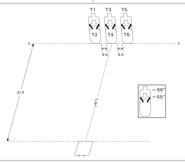
**SETUP NOTES:** Targets are set at 31 feet from the front of the shooting box, and are spaced 9 inches apart, edge to edge. The shoulders of T1, T3, and T5 are at 66 inches. The shoulders of the no-shoots are at 55 inches. Set the top edges of T2, T4, and T6 at 7.5 inches below
