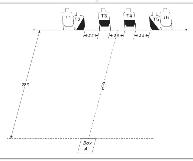
**SETUP NOTES:** Set T1, T3, T4, and T6 to 5 feet high at shoulders. T2 and T5 are set so top of upper A zones are parallel with top of shoulder on adjacent target. Outer non-scoring edges of T1-T2 and T5-T6
