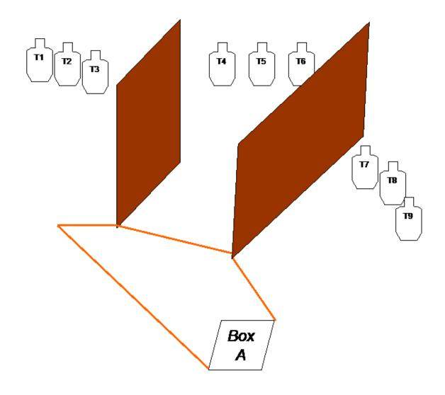
**SETUP NOTES**: Setup in Right corner of Right bay. Set T7-T9 back far enough to avoid a 180° trap. Spread out the arrays to avoid having a sweet spot to shoot all 3 arrays from one location. T4-T6 should be in the corner.
